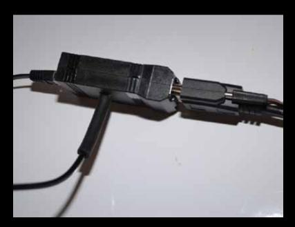
Connect the vacuum line and harness to the control box as shown. (note: for versions earlier than 2.1, the vacuum port is on the harness)
