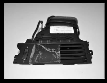
If you ordered a model pre-installed into the vent, then you are ready to install into the car. If you did not purchase the gauge pre-installed, assemble the vent gauge into the vent. Download vent install instructions from
