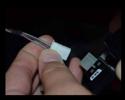
**(Optional)** To use the auto dimmer, D.On.A function of the gauge, connect the GREEN harness wire to the Red/Gray wire on the TRUNK POP SWITCH with the T-Tap connector. If you do not tap this wire for dimmer, you can use the one-touch manual dimmer option on the gauge.
