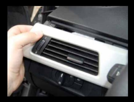
With the driver's door open, remove the vent from the car with trim attached.
