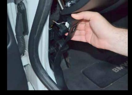
Flex this panel forward to get access to the OBD2 port and the trunk pop switch. You will need to pull the rubber door seal forward to free the panel.
