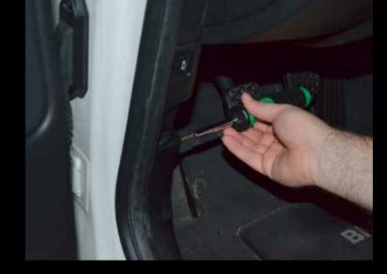
Remove the side kick panel cover screws, first remove the Phillips screw holding the hood pop lever, then the screw behind the lever. 2 screws total.
