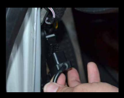
Plug in the obd2 connector to the car.
