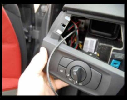
Remove the light switch assembly to give yourself room to work, it just pulls out.
