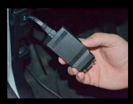
Feed the display wire down to the lower dash footwell area and connect it to the control box.
