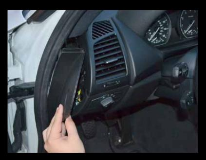
Remove the side dash cover as shown. It is easiest to start at the bottom of the panel first.
