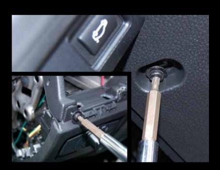
Remove the light switch panel by removing two #20 torx screws at the top, and one at the bottom as shown.
