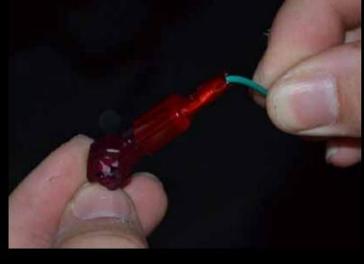
(Optional) To use the auto dimmer, D.On.A function of the gauge, connect the GREEN harness wire to the Red/Gray wire on the TRUNK POP SWITCH with the T-Tap connector. If you do not tap this wire for dimmer, you can use the one-touch manual dimmer option on the gauge.
