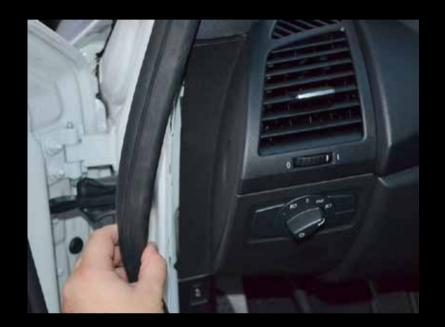
With the driver's door open, pull off the rubber door seal, it is just a friction fit. Now we have access to the edge of the dash and kick panels.
