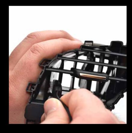
Insert the wire in the vent by squeezing the connector through the left bottom corner as shown. Feed all the wire through.
