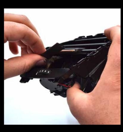
Now remove the second from bottom slat, this slat will have a small metal controller bar behind it that will need to unhook from the slat above it as it comes out. Once again, take care that the other slats do not come out.
