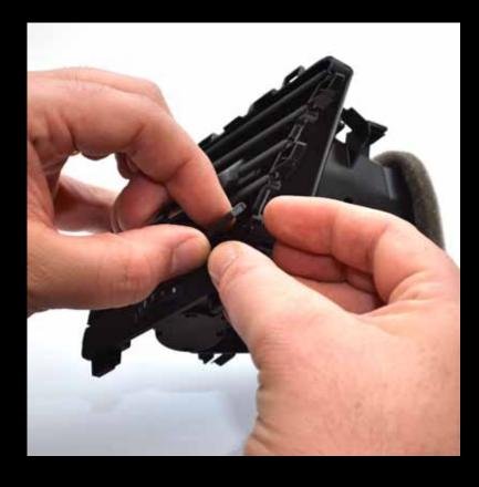
Carefully remove ONLY the bottom slat starting on the side of the vent that is closest to the steering wheel.
