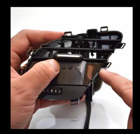
Peel the protective covering off both sides of the glass face so the tabs are not covered. Insert the tabs on the glass into the holes on the vent as shown here starting with the far side. The gauge should rest inside the slots where the vent slates were before. If the gauge will not sit flush, check that the wire is positioned properly.
