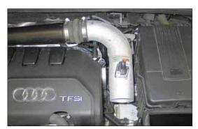
24. Install the K&N secondary intake tube into the silicone hose at the factory intake tube and secure with the provided hose clamp.
