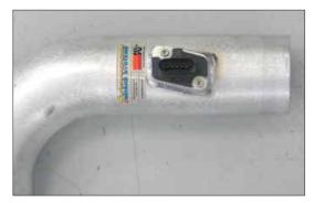
23. Install the mass air sensor into the K&N secondary intake tube and secure with the provided hardware.
