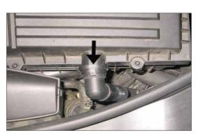
3. On vehicles equipped with an air injection system, release the air injection hose coupler from the upper air box half.
