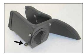
19. Install the heat shield mounting bracket (010051) onto the heat shield using the provided hardware.
