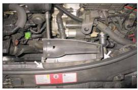
11. Remove the two screws which secure the fresh air inlet duct to the core support and then remove the duct from the vehicle.
