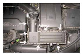
4. Loosen the eight screws securing the upper air box to the lower air box.
