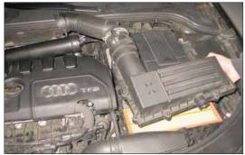
6. Remove the upper air box assembly from the vehicle as shown.
