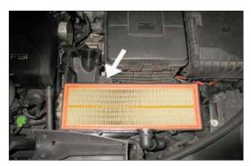
9. Loosen the bolt securing the lower air box to the vehicle.
