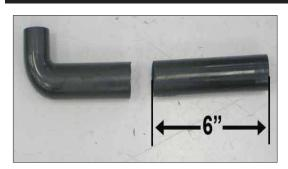
25. On vehicles equipped with an air injection system, cut 6" off of the provided air injection hose as shown.
