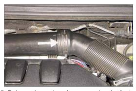
5. Release the spring clamp securing the factory intake hose to the factory intake tube and then unhook the intake hose.
