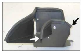
16. Install the 11" length of edge trim onto the heat shield assembly as shown.
