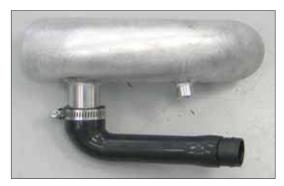
27. Install the air injection hose assembly onto the K&N primary intake tube as shown and secure with the provided hose clamp. On vehicles not equipped with air injection, install the provided cap plug onto tube and secure with the provided hose clamp.
