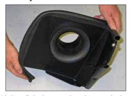
13. Install the longer edge trim onto the heat shield as shown.
