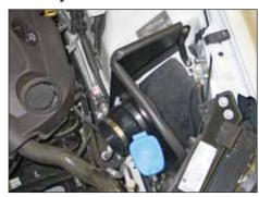
14. Install the heat shield assembly into the vehicle and secure with the factory nut from step #6 and hardware provided.
