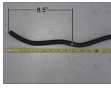
24. Measure 8.5' from the end of the tube and then cut the tube using a sharp knife.
