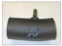
17. Install the  $\frac{1}{4}$ "npt vent fitting into the K&N® intake tube as shown.
