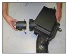
15. Remove the mass air sensor from the factory air box.
