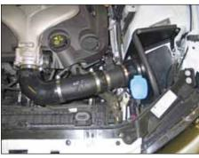
20. Install the intake tube assembly onto the throttle body and mass air sensor, adjust for proper fit then secure with the provided hose clamps.
