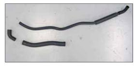
23. Remove the elbow and foam insulation from the crank case vent tube as shown.
