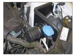
16. Install the mass air sensor onto the heat shield assembly and secure with the provided hose clamp. NOTE: Be sure to correctly position the mass air sensor in the correct direction as indicated by the arrow which shows the way of air travel.
