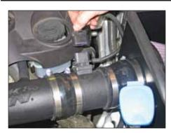
29. Reconnect the mass air sensor electrical con-
