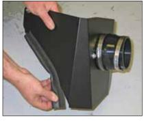
12. Install the shorter edge trim onto the heat shield as shown.
