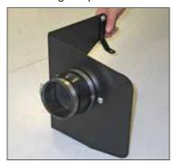
11. Install the provided silicone hose (08050) onto the filter adapter and secure with the provided hose clamp.
