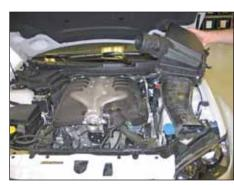
7. Pull up firmly and remove the air box from the vehicle.
