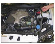
22. Disconnect the crank case vent tube from the valve cover and remove from the vehicle.
