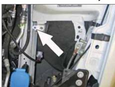
8. Remove the lower air box mounting stud shown.
