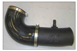
18. Install the angle hose (084089) onto the K&N<sup>®</sup> intake tube and secure with the provided hose clamp.
