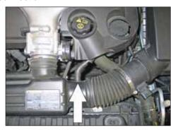
3. Disconnect the crank case vent line from the factory intake tube.
