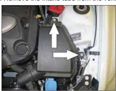
6. Remove the two nuts which secure factory air box to the inner fender.
