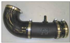
19. Install the silicone hose (08051) onto the K&N<sup>®</sup> intake tube and secure with the provided hose clamp.
