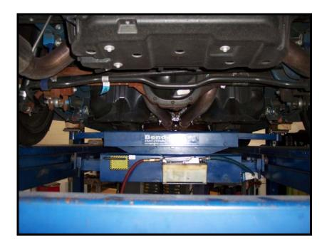
2. Unbolt the lower strut bolt on the slightly raised side. You May need to disconnect the sway bar end link for access to the lower strut bolt.
