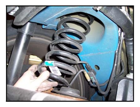
5. Install the new Hotchkis coil spring.
