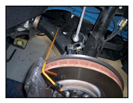
7. Now remove the four (4) upper mounting nuts for the strut. Just before removing the last nut, support the strut to ensure it from not falling.
