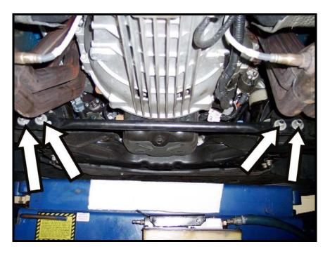
2. Install the new under brace by hand tightening the four (4) nuts/bolts. If only holes are there use supplied 12mm X 30mm bolts, nylock nuts, and washers. *NOTE: Do not tighten these bolts yet. Just start the bolts in the holes so that the brace is supported. This will make it easier to bolt up the rear section.*
