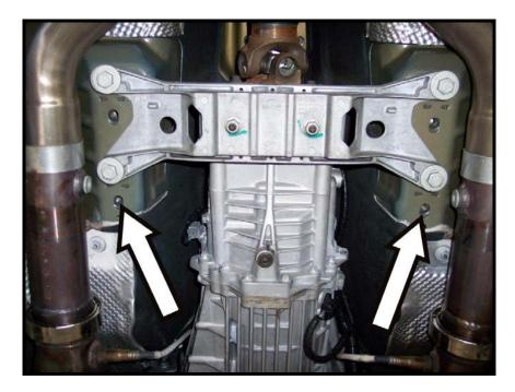
4. Fully tighten the two (2) rear mounting bolts and the four (4) front mounting nuts/bolts and you are finished.
