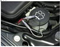
**3e)** Route the long harness across the top of the engine and secure it over the OEM wire holder. See pictures below.
