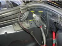
**3c)** Route the short harness to the passenger side headlight. If you lift the weather stripping from the passenger side power terminal area, you can slide the harness under the factory harness bundle then route it down the passenger fender to the passenger headlight.
