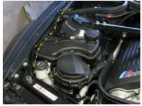
3d) Connect the black rectangular igniter ballast box to the harness (pictured below) and also to the passenger side Angel Eyes (not pictured). Do not mount (tape) the igniter box just yet.
