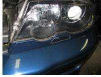
**1d) Remove the clear headlight cover lense.** Tools aren't really necessary here. There are three plastic tabs on top, one on the side, and three on the bottom that must be unlatched. Carefully pull up on each tab till it releases from lense. As you work your way around each tab you should be able to remove the lense by sliding it out.
