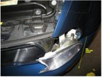
**1b) Remove the rubber trim surrounding the top/side of your headlight.** You can easily undo the top 3 tabs with your fingers by lifting the tabs from behind. The two tabs on side might be easier with a flat head screw driver.
