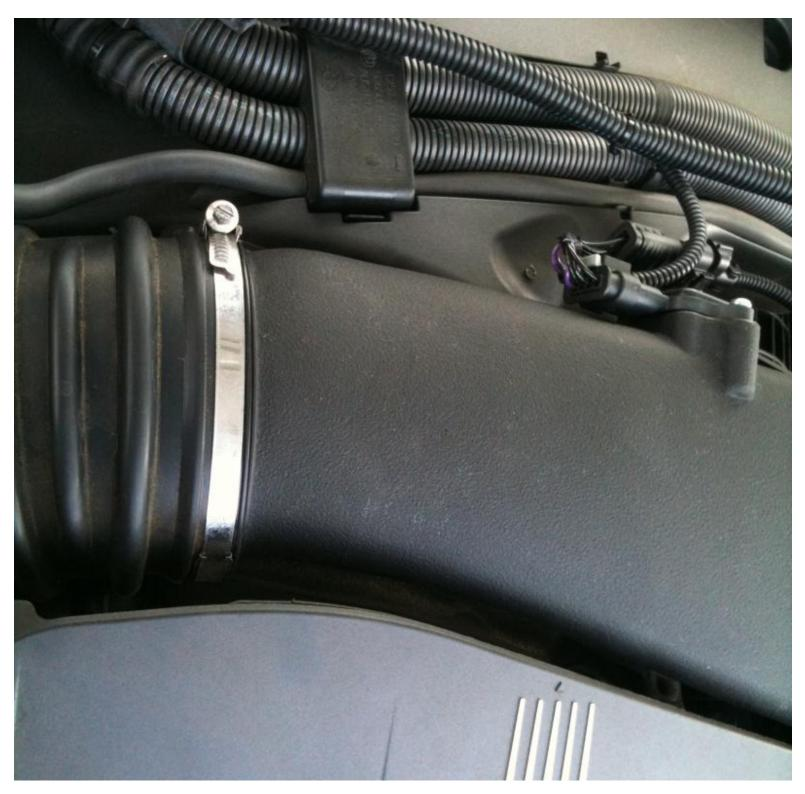
Step 6: Slip the included bracket under the OEM airbox fitting as shown and then tighten to the intake holding it in place. The bracket is designed to allow fine adjustment of the intake position before tightening it down.
