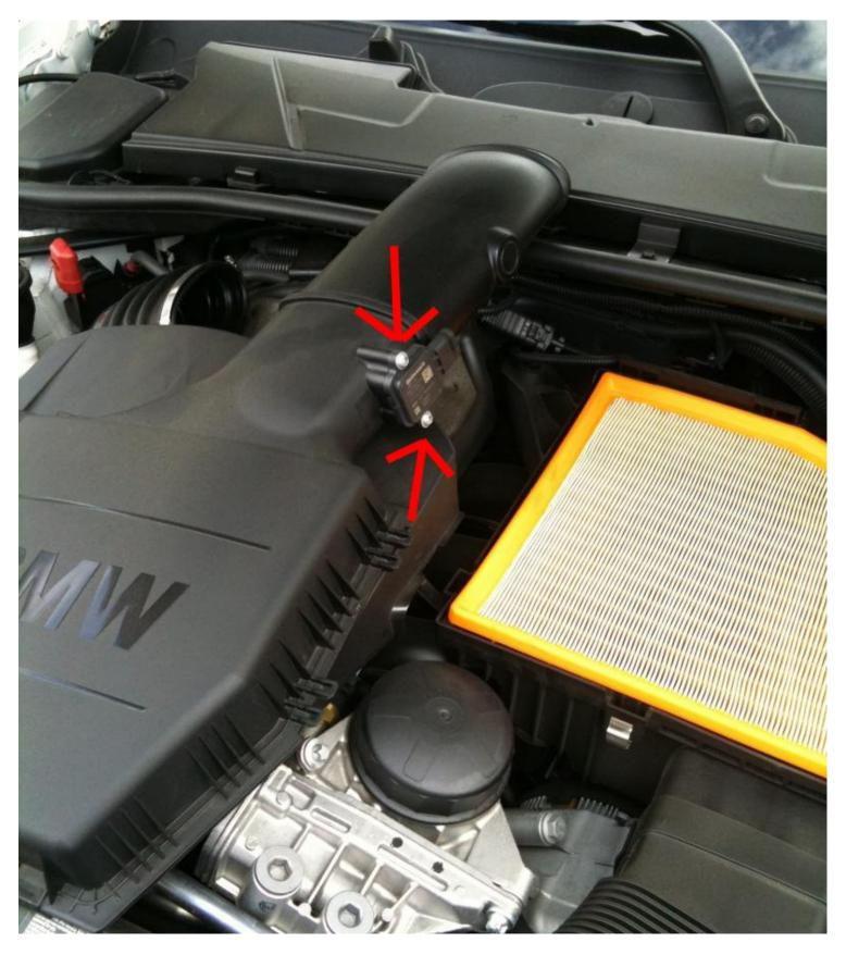
Step 3: Insert the MAF sensor in to the BMS intake and tighten the included screws holding it in. They should be snug but not over tightened. Attach the air filter to the tube and tighten the included hose clamp using a screw driver or an 8mm socket.
