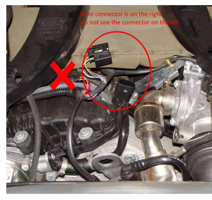
Insert the JBD male connector in to the OEM female connector as shown. Take care to ensure it is fully inserted and the retaining clip closed over the tab.
