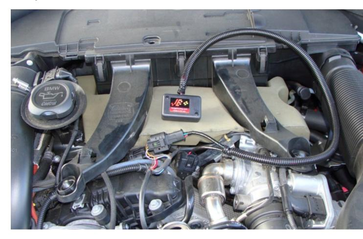
Once connected route the JBD harness to the driver side of the engine bay as shown and secure with a zip tie, twist tie, or simply shove it in a corner.
