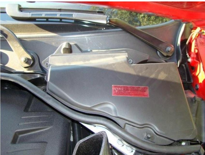
2. Remove the passenger's side air conditioning filter cover. The passenger's side filter cover is the same shape as the driver's side filter, and is also held on by the same three 8mm-hex screws.
