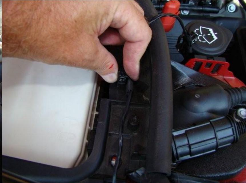
3. Remove the rain gutter tray. This tray is located underneath the two air conditioning filter covers removed in (1) and (2) above. The tray runs the entire width of the engine compartment. The tray is held on by two 8mm-hex machine screws.
