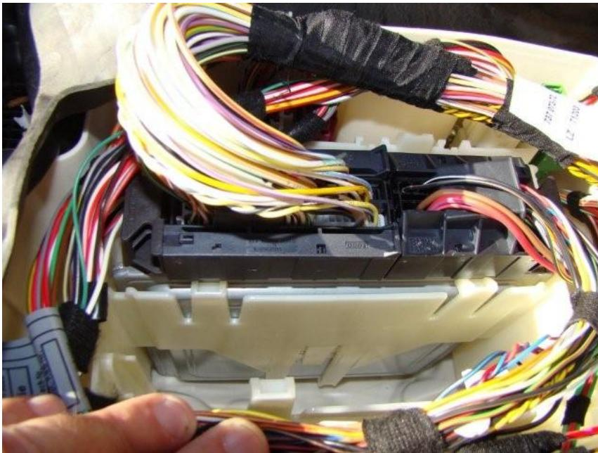
5. Remove the ECU wiring harnesses. Each ECU wiring harness is held in place by a sliding lock. Pull each sliding lock and remove the wiring harnesses.
