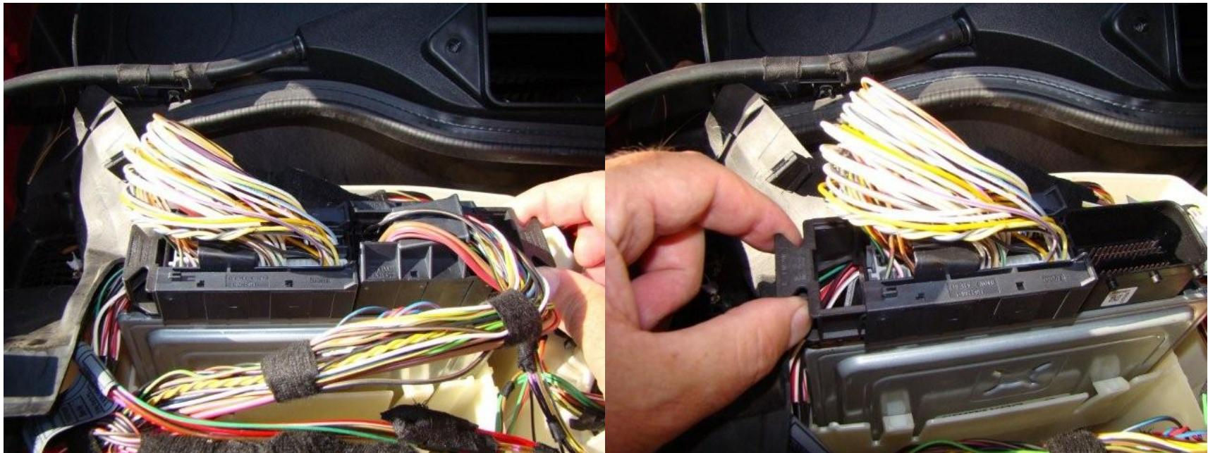
6. Remove the ECU. The ECU is held in by two plastic tabs. Pry these tabs loose, and remove the ECU.
