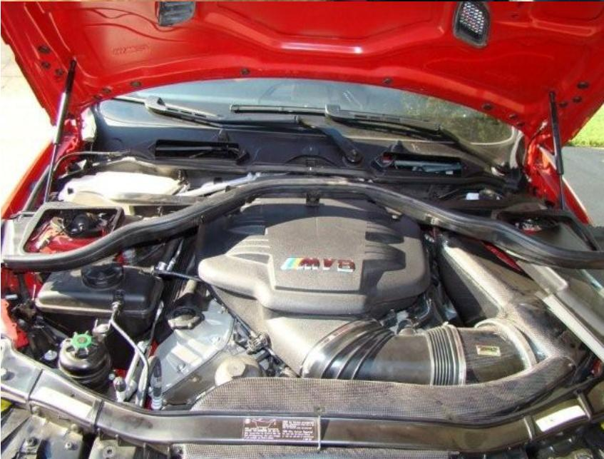
4. Remove the white ECU compartment cover. This cover is held on by two sliding locks, and four locking tabs.
