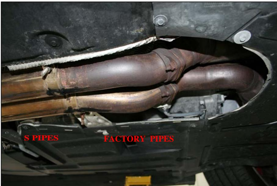
Shown with Factory pipes cut and "S PIPES" installed
