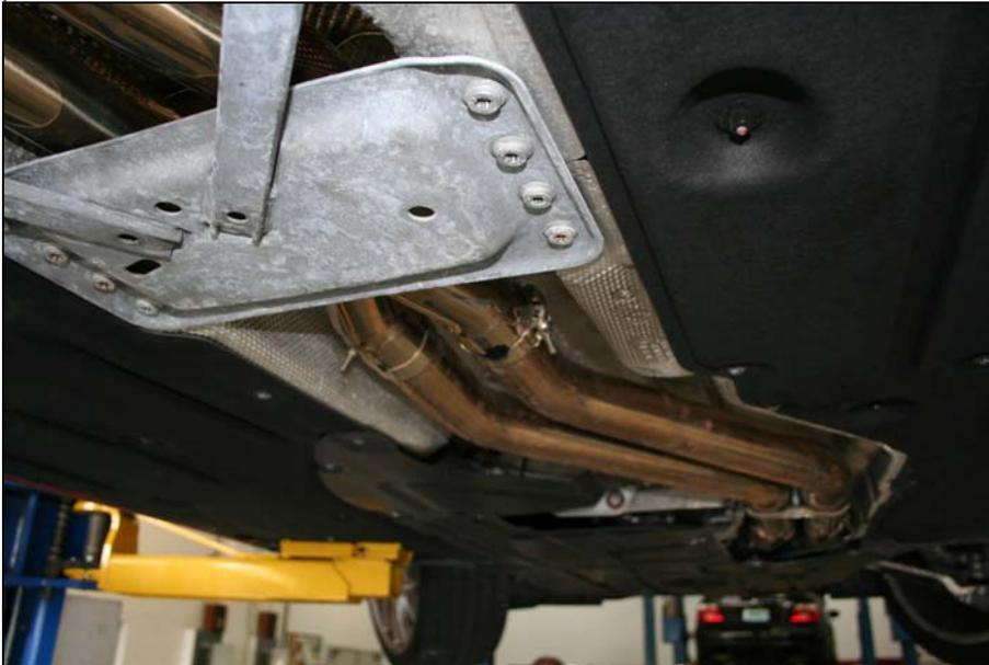
View of "S PIPES" installed
