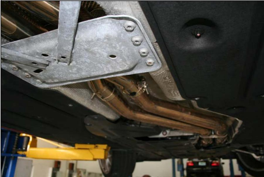
View of "S PIPES" installed
