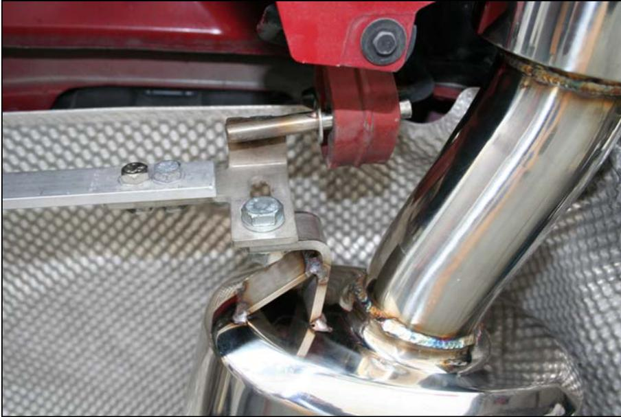
Mount rear mufflers to MUFFLER REAR BAR
