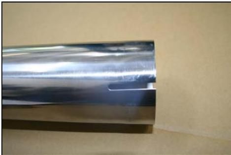
SLIT in pipes for proper compression
