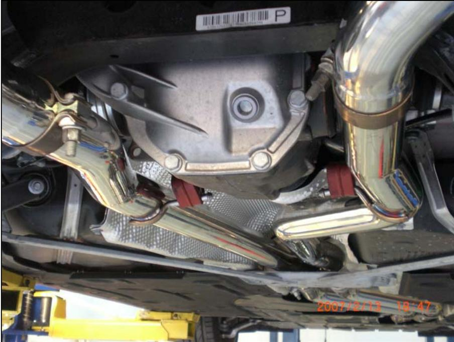
A rear view of "X PIPE" installed
