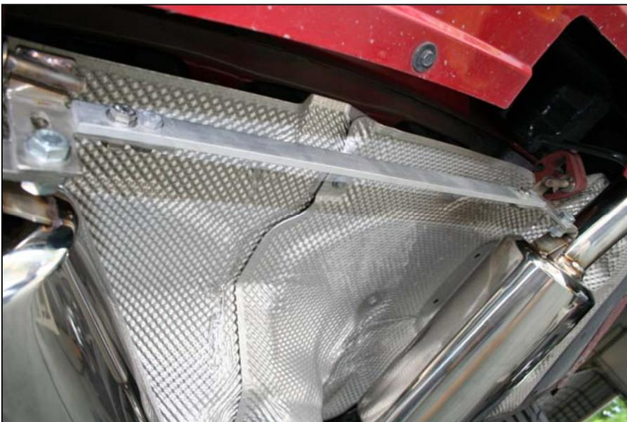
With Muffler REAR BRACE installed, it makes for a much easier installation of the rear mufflers later
