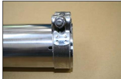
Proper position of CLAMP over slit opening
