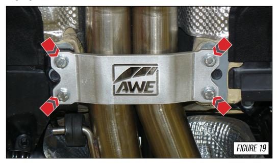
With everything installed onto the car, you are ready to adjust the exhaust and begin the final torque procedure. Minimum torque specification for the Accu-Seal clamp is 40 ft.lbs.
