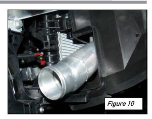
Connect the factory intercooler inlet and outlet hoses and reinstall all the bumper support factory fasteners and clips.
