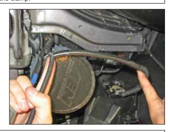
o. Install the supplied section of wire loom on the exposed fog light wires and secure it with tape. Unclip the washer fluid hose from the clip that attaches it to the inner fender, and push the hose and two wire connectors up top behind the headlight.
