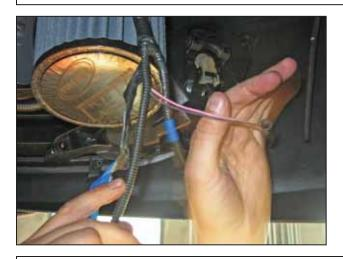
n. If the vehicle is equipped with fog lights, unwrap the wire loom as shown and separate the fog light wires.
