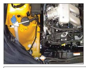
e. Remove the M6 bolt securing the washer bottle neck and unplug the right headlight.
