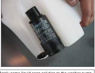
c. Apply some liquid soap solution to the washer pump and insert it into the grommet. Firmly press the pump all the way into the grommet.
