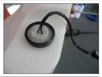
e. Apply liquid soap solution to the level sensor and insert it into the grommet. Make sure that the level sensor is pressed all the way into the grommet. The lip of the sensor should be inside the grove of the grommet.
