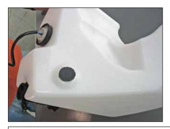
f. Apply the self adhesive rubber pad onto the protrusion on the underside of the washer bottle as shown. Set the new washer bottle assembly aside.
