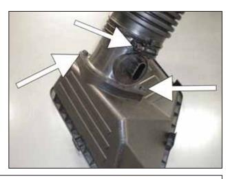
g. Disassemble the MAF from the airbox by removing the two screws. Also loosen the clamp securing the rubber inlet hose to the MAF and remove the hose.
