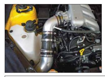
I. Install the lower pipe with the 4.0" x 2" coupler and two #64 clamps. Align the bracket with the rubber mount and secure it with the washer and M6 nut.
