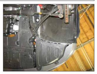
q. Reinstall the fender liner and wheel.
