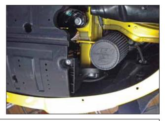
m. From underneath the car, install the filter with the #64 clamp. Slide the filter onto the end of the pipe until the pipe reaches the stop inside the filter, then tighten the clamp.
