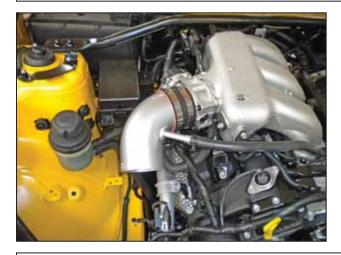
h. Install the upper pipe and 3.5" x 2" throttle body coupler as shown with two #60 Clamps. Secure the crankcase vent hose to the nipple on the inlet pipe with the OE spring clamp. Plug in the headlight unplugged in Step 2e.
