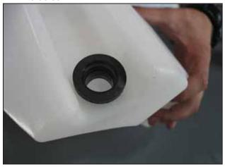
b. Insert the stock washer pump grommet into the hole on the front of the supplied washer bottle.
