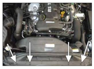
a. Remove the four clips securing the air scoop, remove the air scoop from the vehicle.
