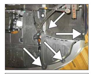
u. Reinstall the inner wheel liner with the three clips and one screw removed in step 2f.
