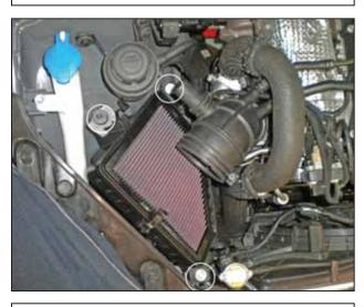
c. Remove the three M6 bolts securing the lower air box, then remove the lower air box.
