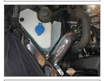
s. Refill the washer bottle with the washer fluid drained in step 2h. Snap the blue cap onto the neck of the washer bottle.
