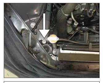
c. Install the M6 rubber mount in the location shown.
