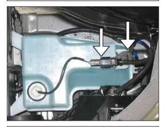
g. Unplug the washer pump and washer fluid level sensor.
