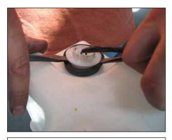
I. Using two flat head screwdrivers, carefully pry up on the lip of the washer level sensor, using care not to damage the rubber grommet. A soapy water mixture may be used to aid with the sensor removal. Also, remove the grommet and set aside in a safe area.
