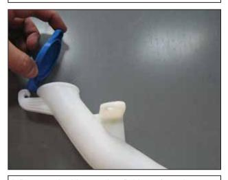
i. Remove the blue washer fluid cap from the stock washer bottle neck.
