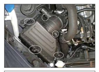
b. Loosen the hose clamp on the inlet hose. Unclip the four clips on the air box top and remove it from the vehicle.
