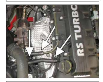
d. Loosen the hose clamp at the compressor inlet. Locate the two breather hoses connected to the valve cover inlet nipples, compress the spring clamps and slide them off the inlet nipples so the hoses can be removed.
