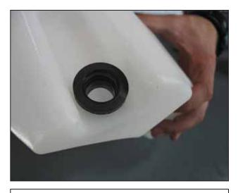
m. Insert the stock washer pump grommet into the inlet on the front of the supplied washer bottle.
