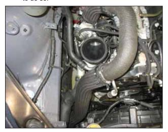
b. Install the compressor inlet coupler using a #9456 and #9444 hose clamp; orient as shown. Plug in the headlight that was unplugged in step 2e.
