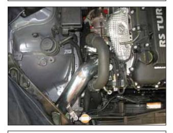
d. Install the inlet pipe by lowering the front end into position, then insert the rear end into the compressor inlet coupler. Guide the pipe's bracket into position on the rubber mount and secure with a M6 nut and washer. Leave the M6 nut loose for now.
