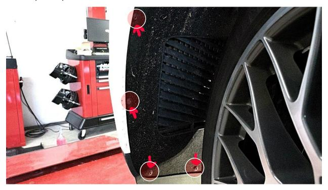
) Once the fender liner is pulled back you will see a black bracket. There are 2x T25 screws that are tucked into 2 pockets. Remove the 2 screws. Repeat on the other side.
