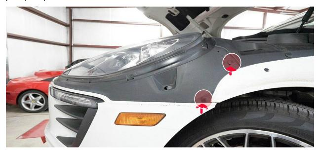
**5)** With the plastic panel removed, you have access to 2x T25 screws. Remove these. Repeat on the other side.
