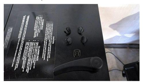
Remove the screws holding the top of the bumper. There are 2x T25 torx screws and 2x T27 torx screws. The T25 screws are the ones on the outside and the T27 screws are the 2 on the inside. The T27 screws are reverse thread and will not fully remove from the bumper. Notate how far the T27 screws are screwed in for reinstall.
