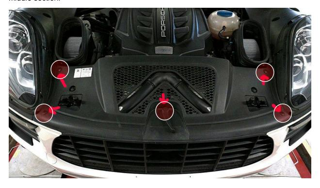
2) Remove the hood latch handle. To do this you need to remove a slide clip that is holding the handle in place then wiggle the handle back and forth as you pull up. Not much force needs to be applied but it might be a little tight. Remove plastic panel and set aside.
