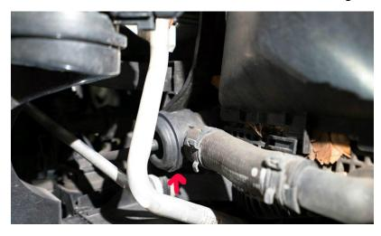
12) Install the valves the same way you removed them. Reuse the factory vacuum line and all hosing. You may want to dab a tad bit of oil on the housing to allow for an easier entry of the diverter valve.
