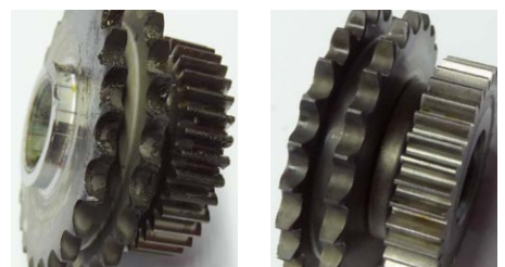
Removal of grease and silicone
