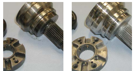
Removal of oxidation and other contaminants
