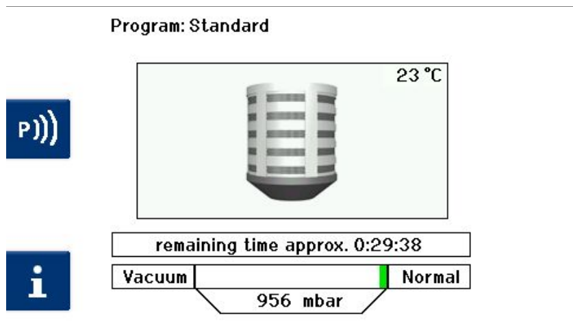
Fig. 6.3.4 Display Status of the program progress
