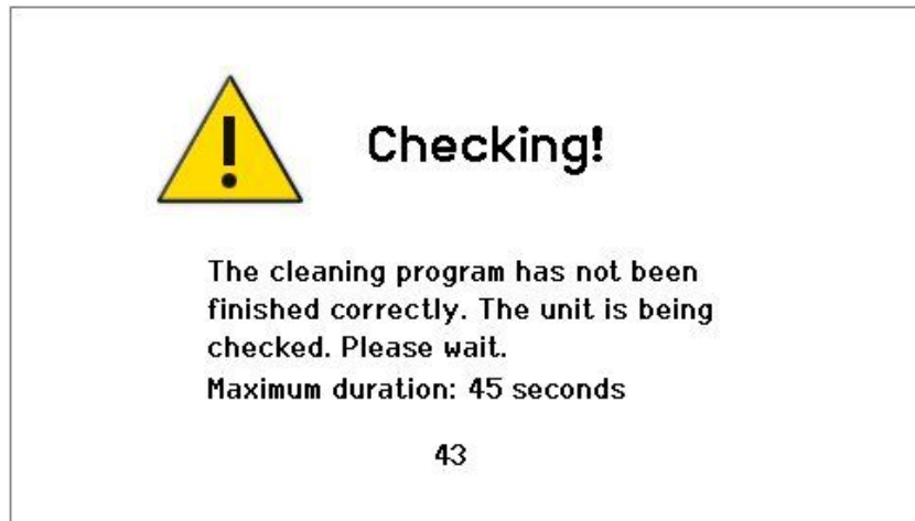
Fig. 11.1.2 Fault information for cleaning machine checking
