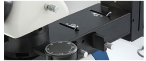
Bertrand lens, \lambda Slip, 360° rotatable analyser (removable)
