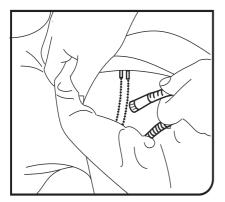
3.3 Open the zip in the inner bib so that the Cable from the Head Set can pass though.
