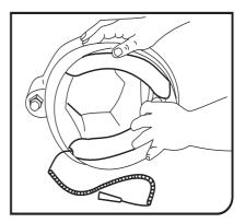
3.2 Place the Nova Talk Sidewings into the helmets, ensuring that they are securely attached to the Velcro Studs .
