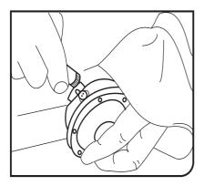
2.5 Connect the PTT cable to the head set cable and place the cable underneath the cape.
