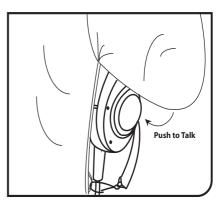
2.6 To operate the device, press your elbow onto the PTT Button, and then speak.
