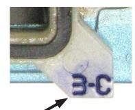
When valve is configured incorrectly, "C" will be showing on tab.
