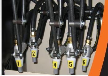
Six or Four Blast Guns mounted on separately adjustable holders enable operators to control blast coverage.
