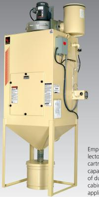
Empire's CDC-12 dust collector features quick-change cartridge filters and high capacity. We offer a variety of dust collectors with IL-885 cabinets to suit specific application requirements.
