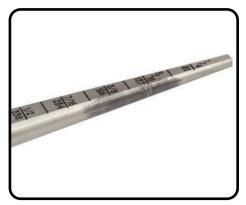
STEP 4: Remove the gauge and locate the mark <u>closest to the handle</u> where the nozzle rubbed off the marking pencil/crayon. This is the current ID of the nozzle bore.
