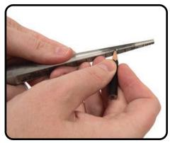
STEP 2: Color in both sides of the gauge starting at the original size of the nozzle, and several sizes larger.
