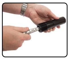
STEP 3: Insert the gauge into the threaded/inlet side of the nozzle until it stops and give it a couple of turns.
