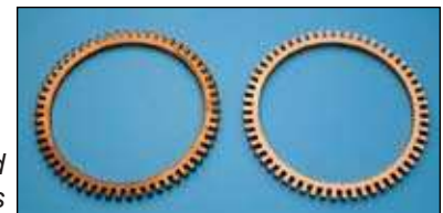
Collar deburred with glass beads
