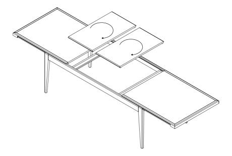
Place the loose tops on the frame and close the sliding tops.
