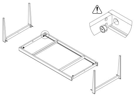
Insert the legs all the way in, then tight the disc, which must pull the insert towards the frame.
