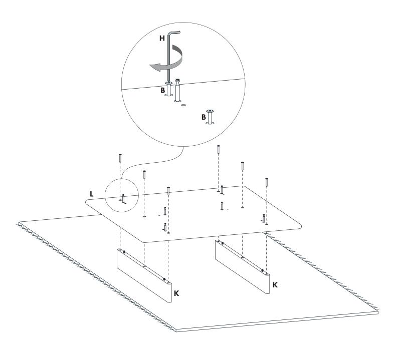
FIX THE UPPER FRAME TO LOWER FRAME AND TIGHTEN THE GRUB SCREWS BY USING A SCREWDRIVER.
