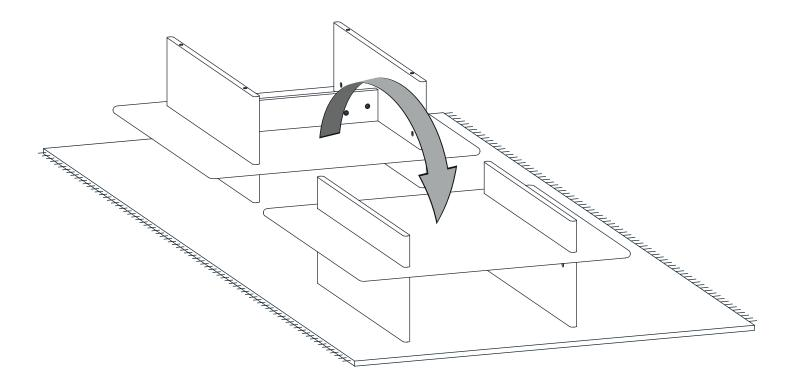
REMOVE THE PROTECTIVE PAPER FROM THE SILICON BUMPER AND ATTACH THEM TO THE TOP OF VERTICAL SUPPORTS.
