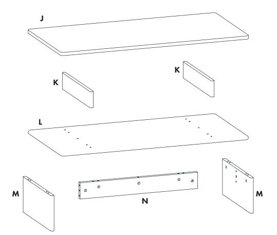
PLACE THE WOODEN DOWELS TO THE LEG PANELS, VERTICAL SUPPORTS AND CROSS RAILS BY USING A SOFT MALLET.
