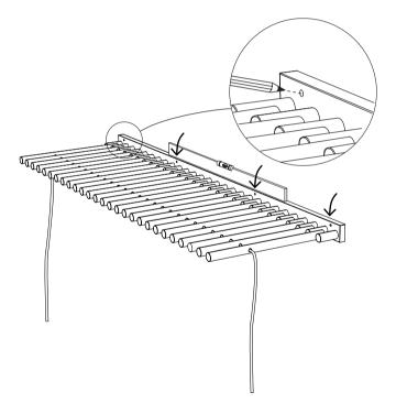
DRILL FOUR HOLES IN THE WALL AT THE MARKED SPOTS
