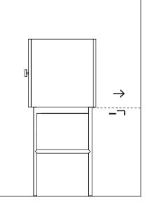
MEASURE THE HEIGHT AND DRILL HOLES IN THE WALL APPLY WALL PLUGS THAT ARE SUITABLE FOR YOUR WALL. MOUNT THE METAL BRACKET TO THE WALL WITH SUITABLE SCREWS AND THEN MOUNT THE BRACKET TO THE CABINET.
