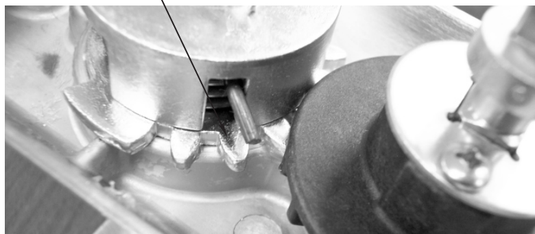
Spring orientation for right hand reverse operation
