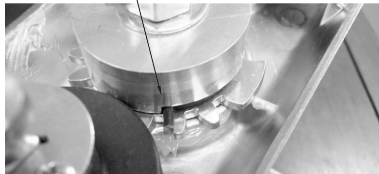
Spring orientation for right hand reverse operation
