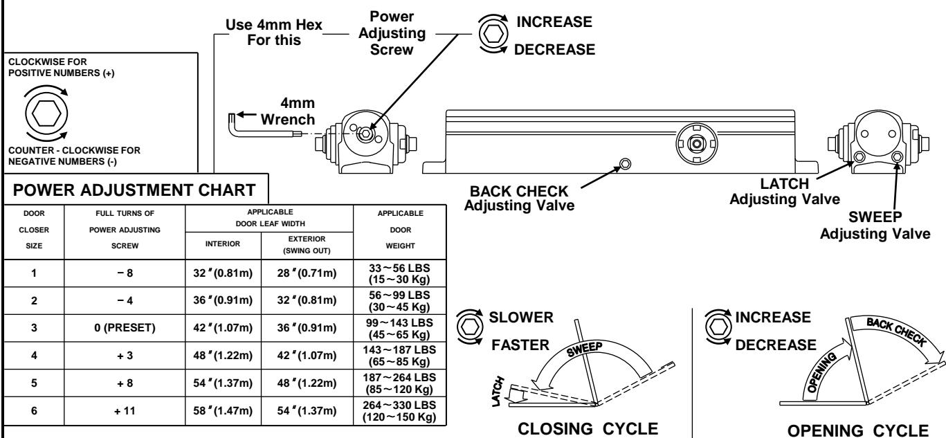
**CAUTION!!** Do not turn speed adjusting valve more than two(2) full turns counter-clockwise. Do not back valves out of closer or a leak will result.
