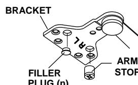
**FOR RIGHT HAND DOOR:** Remove filler plug from bracket. Using the phillips screwdriver turn the REMOVABLE ARM STOP counter-clockwise to remove it. Insert REMOVABLE ARM STOP into hole mark "R" and using the phillips screwdriver, turn clockwise to seat as tightly as possible. Push filler plug into the other hole firmly.
