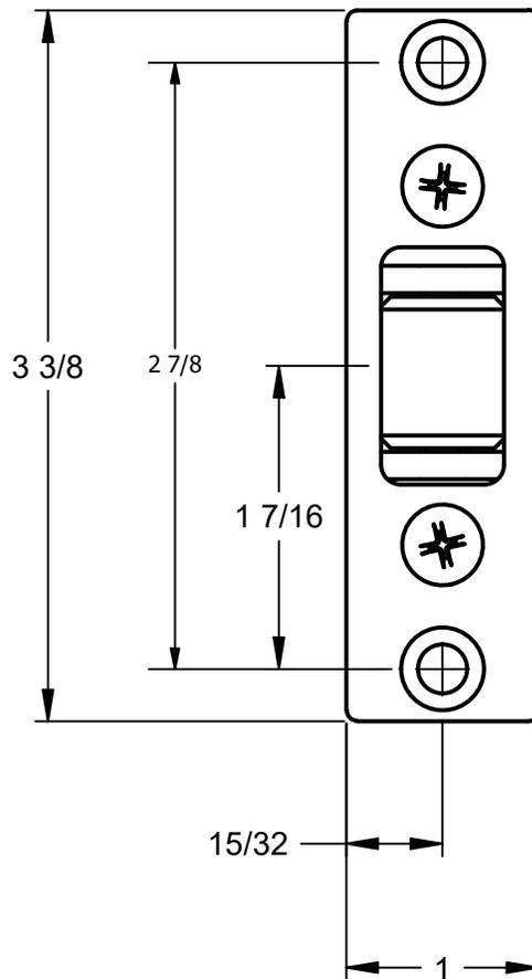
SUPPLIED WITH TWO (2) #10 X 1-1/4 FLAT HEAD, PHILLIPS DRIVE WOOD SCREWS
