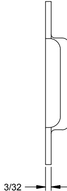
SUPPLIED WITH TWO (2) #8 X 1 FLAT HEAD, PHILLIPS DRIVE WOOD SCREWS
