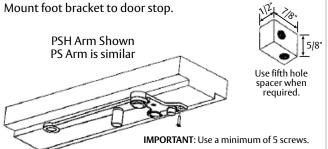
3A. Alternate Option: Pre-assemble arm prior to attaching stop.
