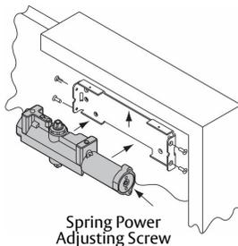
Drill & Tap, use screws provided or use Mortise Nuts when required.
