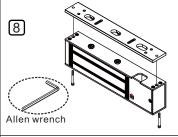
Attach the magnet to the mounting plate. Use the Allen wrench and thru-bolts to tighten the magnet to the mounting plate.
