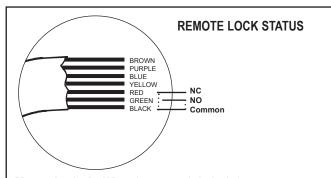
**Magnet Locked** – When the magnet is locked, the common contact (black) and the normally open contact (green or white) are closed. The normally closed contact (red) would be open.
