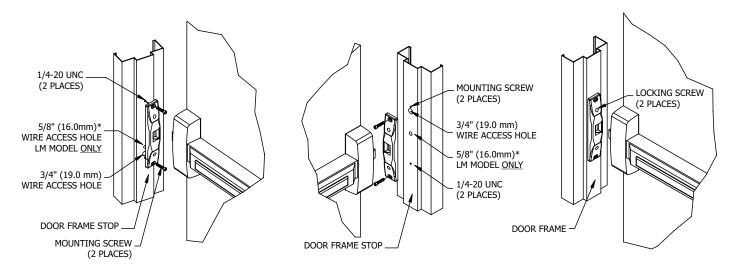
**NOTE:** Wire access hole locations are relative to the exit device orientation. **NOTE:** \*Second wire access hole required for 0162LM only **NOTE:** Not to scale. Specifications are subject to change without notice.
