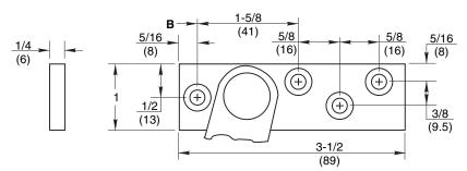
3. Locate "A" and "F dimensions on centerline of door and mortise 1-5/8" (41mm) deep for channel. 1/16" (2mm) head clearance shown. Coordinate the arm and rail cutout dimensions if head clearance varies.
