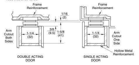
4. Locate "C" and "E" dimensions on top of door and mortise 3/8" (9.5mm)deep as shown for arm cutout.
