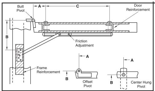
5. Install channel on door with "A" dimension sex bolt. Locate "C" dimension sex bolt hole making sure that channel is horizontal and parallel with stop strip. Drill 5/16 (7.9) dia. sex bolt hole and finish installing holder.
