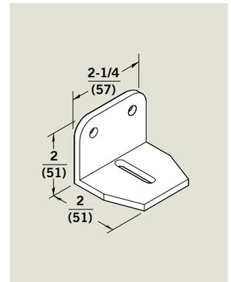
**NFHD** — For use with all 8900 Series DS and SPA applications where total frame depth is less than 4-1/2" (114 mm), prohibiting use of standard spacer block. NFHD bracket is in lieu of block supplied with arm.
