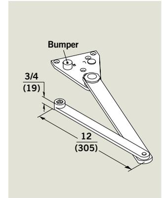
Heavy-duty parallel arm with integral cushioned opening function. Available in non-hold open, thumb turn hold open, and hex key turn hold open. Units can be installed to achieve either stop or stop and hold open at 85°, 90°, 100°, and 110°. Maximum opening is 110° (conditions permitting). Arm is non-handed. Non-hold open arm illustrated.
