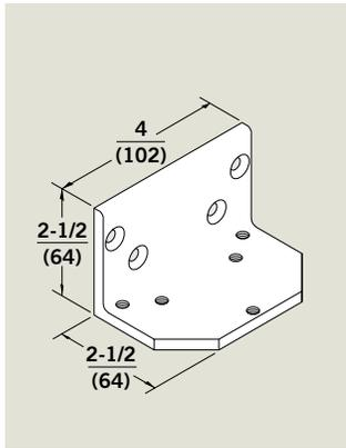
**FTHD** — For use with all 8900 Series DS and SPA applications where flush transom conditions prohibit normal installation of soffit bracket.
