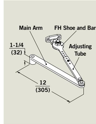
Provides a hold open function between Approx. ly 90° and 180° of door opening (conditions permitting). Arm is non-handed.
