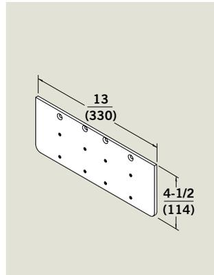
**DP89** — For parallel arm installation of 8900 Series closers when top door rail is less than 5-3/4" (146 mm) for non-hold open and plunger hold open. When top door rail is less than 6" (152 mm) for friction applications (assuming 5/8" (16 mm) stop dimension).
