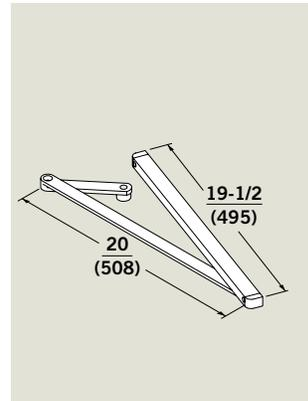
Provides slide track function for pull-side reveal conditions up to 3-1/2". Provides 125° of door opening (conditions permitting). Arm is handed. Also available with hold open option to provide selective single point hold open between 30° and 110°. Arm requires a minimum 3-3/4" clearance between door face and wall when opened 90° and greater.
