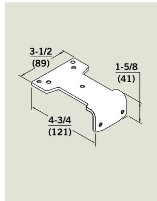
**PHB** — Furnished standard with 8900 FHP Series closer friction hold open parallel arm applications. Spacer block furnished standard for use with narrow stop applications.
