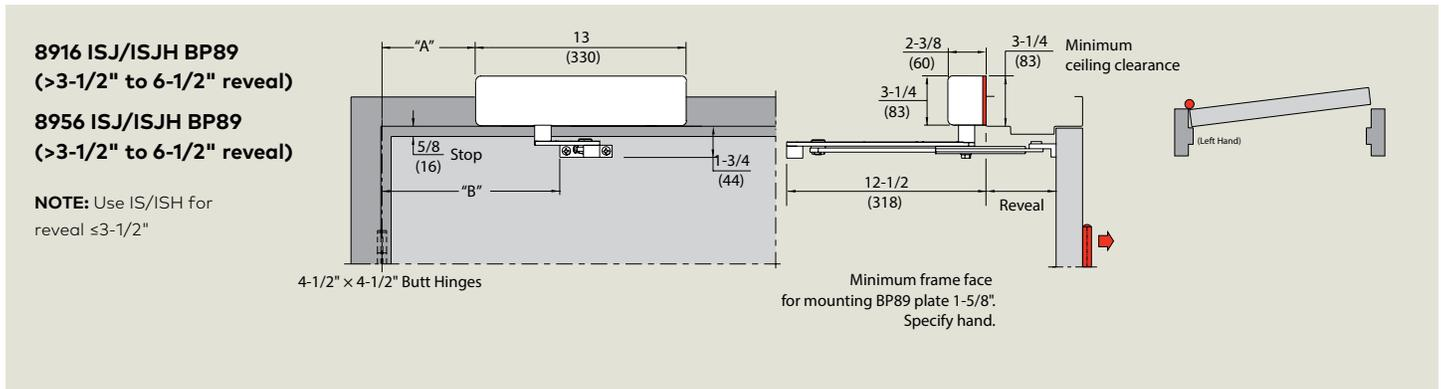
\* Backcheck positioning valve factory preset to on, advancing backcheck approx 15°. **NOTE: Bold type shows supplied arm.**
