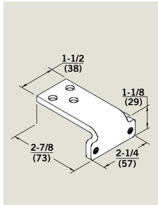
**MJ** — For 8900 Series closers with regular mount non-hold open assemblies where frame conditions will not permit use of the standard foot, e.g. molded, bull nose, or ornate trim. Permits use of parallel arm application between twin communicating doors where limited space prohibits use of P89 bracket. Flat form arm applications must use MJ in combination with AF8MJ Arm.
