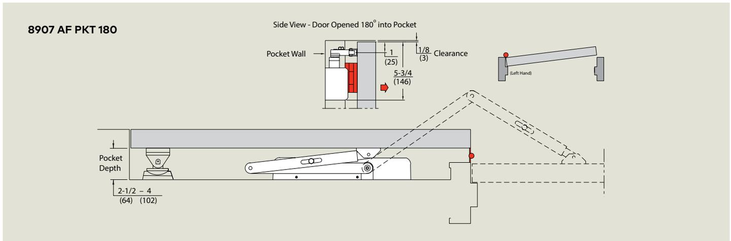
The recommended method for hanging the door is via the use of butt hinges, which create optimum unobstructed space when the door is in the pocket. Alternate methods using 3/4" Offset Pivots, Swing Clear Hinges, or Continuous Hinges are available. When using alternate methods, note where the pivot point of the hinge or pivot locates the door's angle of opening in order to determine the pocket depth.
