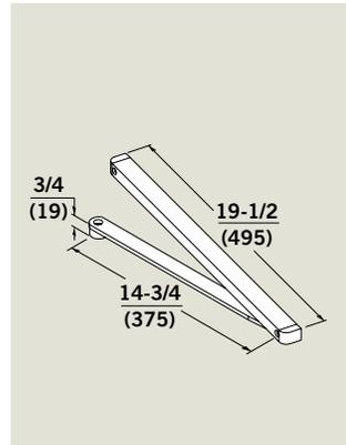
Provides slide track function for improved aesthetics and vandal resistance. Units can be installed to provide 85°, 90°, 110° or 180° of door opening (conditions and application permitting). Arm is non-handed. Also available with hold open option to provide selective single point hold open. Range of hold open and maximum opening varies with mounting application. T version illustrated.
