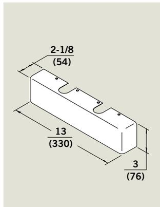
**FMC** — Full metal cover. Specify hand for top jamb, T track, and FT track applications.
