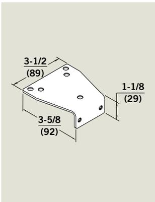
**P89** — Furnished standard with 8900 P Series closer non-hold open and plunger hold open parallel arm applications. Spacer block furnished standard for use with narrow stop applications.
