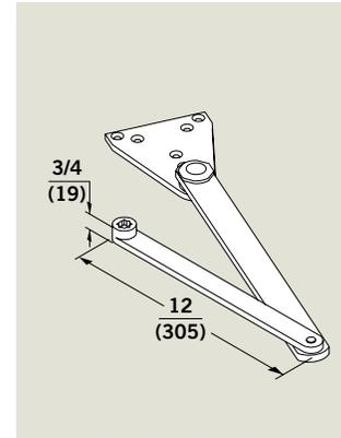
Heavy-duty parallel arm. Available in non-hold open, thumb turn hold open and hex key turn hold open. Units can be installed for maximum opening of 100° or 180°. Hold open units will hold open at 90° or 125°. Maximum opening is 180° (conditions permitting). Arm is non-handed. Non-hold open arm illustrated.
