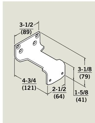
**PFT** — For all 8900 Series closer hold open and non-hold open parallel arm installations where flush transom conditions prohibit use of P89 or PHB bracket.
