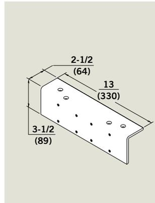
**AB89** — For installation of 8900 Series closers where parallel arm and top jamb applications are not practical due to low overhead ceiling clearance, narrow frame face, or unusual trim conditions. This bracket can also be used to provide clearance for a surface-applied stop/holder.
