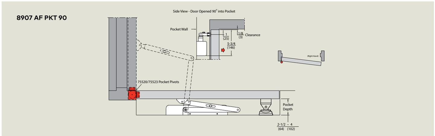
All dormakaba pocket door closers, combined with a dormakaba EM Series wall magnet, create a held open flush door until power is interrupted or the door is manually shut. See EM and LM Series product brochures for specific magnet and pivot information.
