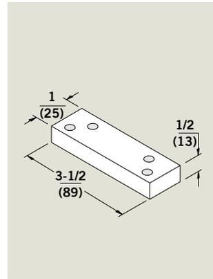
**BS** — For use with all 8900 Series P89, PD, and PHB applications installed on cased frames with applied blade stops. This block is used in conjunction with the spacer furnished with the arm to provide adequate clearance for the blade stop.
