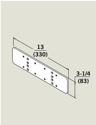
**BP89** — For mounting top jamb when frame face is less than 2-7/8" (73 mm). Two sets of mounting holes accommodate 1-3/4" (44 mm) or 3-1/4" (83 mm) minimum ceiling clearance.\* Top set of holes create top jamb drop application to clear a surface applied stop/holder. Can also be used for regular mount closer to clear mortised stop/holder.
