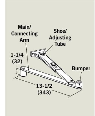
Provides a cushioned opening function for regular and top jamb applications at 85°, 90°, 95°, 100°, 105°, and 110°. Arm is non-handed.
