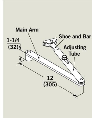
**AF8MJ** — Regular flat form arm complete for use with MJ (mortise jamb) bracket. MJ bracket ordered separately.
