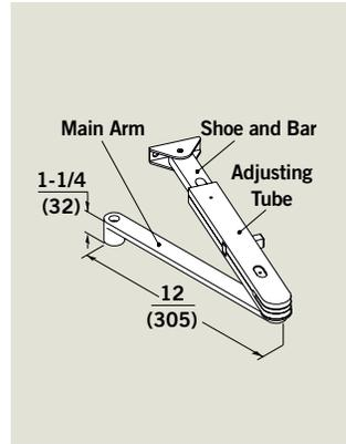
Provides a hold open function at a selected point within a range from Approximately 30° to 130° (conditions and installation applications permitting). Ideal for doors frequently placed in and out of hold open. Arm is non-handed.
