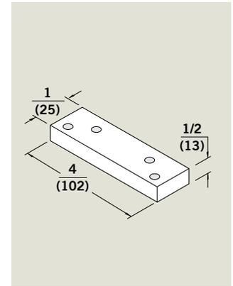
**BSHD** — For use with all 8900 Series DS and SPA applications installed on cased frames with applied blade stops. This block is used in conjunction with the spacer furnished with the arm to provide adequate clearance for the blade stop.
