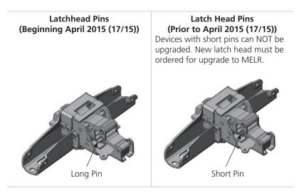
Note: Label with date code is located on front face of latch head.
