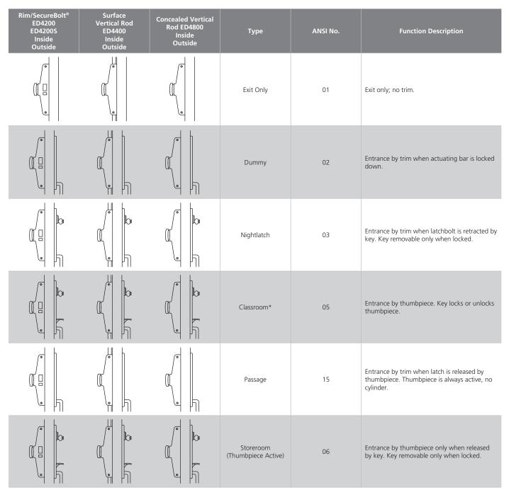
\*Classroom function trims can be converted to Storeroom function by a simple field adjustment.
