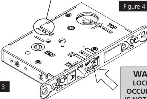
5. Rotate lock front to match bevel of door as shown (Figure 5)
