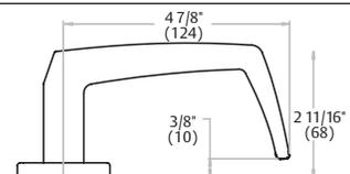
1. Complies with codes requiring lever to return to within 1/2" (13mm) of door face.
