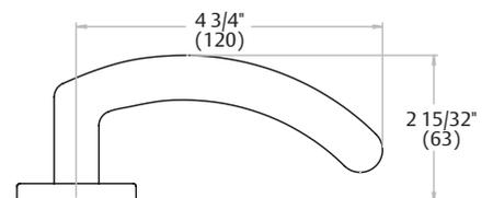
1. Complies with codes requiring lever to return to within 1/2" (13mm) of the door face
