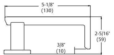
1. Complies with codes requiring lever to return to within 1/2" (13mm) of door face.
