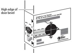
Figure 2 — Placing the template on the high side of the door bevel
