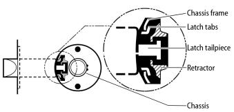
*Figure 5 — Engaging the latch and retractor*
