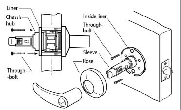
Figure 6 — Installing liner, through bolts, rose, and lever
