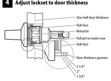
Figure 4 — Adjusting the lock chassis for door thickness
