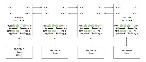
Figure 18. Multidrop configuration ODW-710-F2
