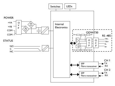
Figure 9. Block diagram for ODW-730-F2
