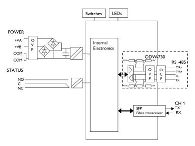
Figure 8. Block diagram for ODW-730-F1
