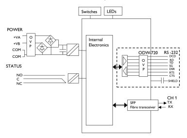
Figure 6. Block diagram for ODW-720-F1
