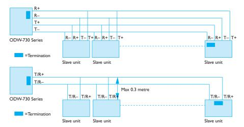
Figure 28. Termination at system level
