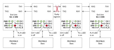
Figure 19. Behavior during optical link failure
