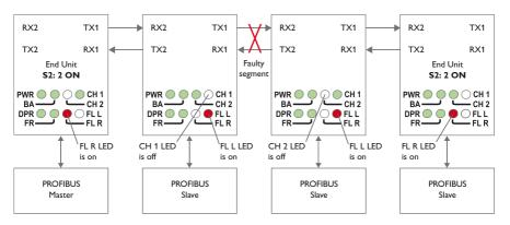
Figure 21. Behavior during optical link failure
