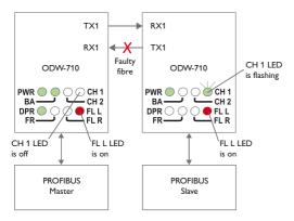
Figure 16. LED indication during optical link failure 1
