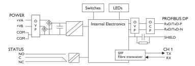
Figure 4. Block diagram for ODW-710-F1
