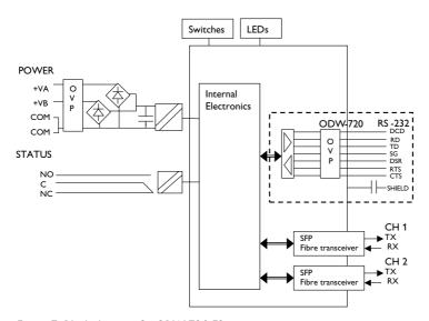
Figure 7. Block diagram for ODW-720-F2
