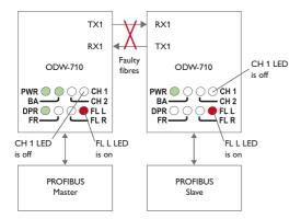
Figure 17. LED indication during optical link failure 2
