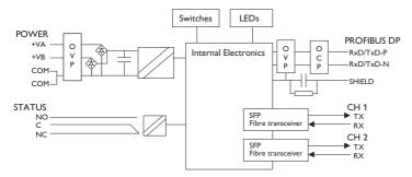
Figure 5. Block diagram for ODW-710-F2
