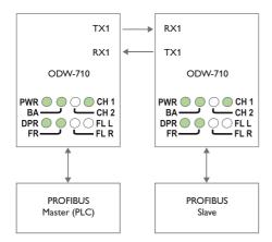
Figure 15. LED indication under normal operation
