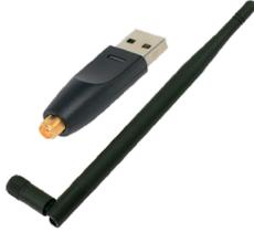
Power OFF the SiteManager and Insert the adapter into a free USB slot, and then power ON.
