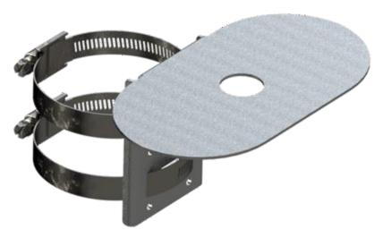
This bracket is designed for smaller antennas needing a 1-inch mounting hole. The included adjustable gear/worm-drive clamps fit poles or rectangular posts with 2.5 to 3.5-inch widths.
