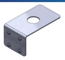
This bracket with a 4-inch-long plate is designed for antennas needing a 1.0-inch mounting hole. L bracket includes predrilled holes and slots for mounting.
