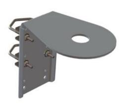
This bracket is designed for antennas needing a heavy-duty mount. This bracket has had stiffeners removed, removing stress concentration points and is twice the thickness of the PTA0149 mount. This Bracket is designed for antennas needing a 1.5-inch mounting hole to securely fit poles with 1.5 to 2.5-inch diameters.
