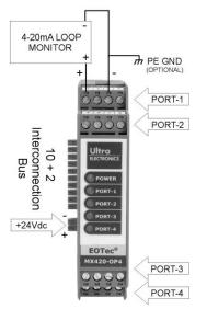
**NOTE:** Internally, this module's negative (-) input terminals are connected to the modules interconnection bus negative (-) terminal (circuit common).
