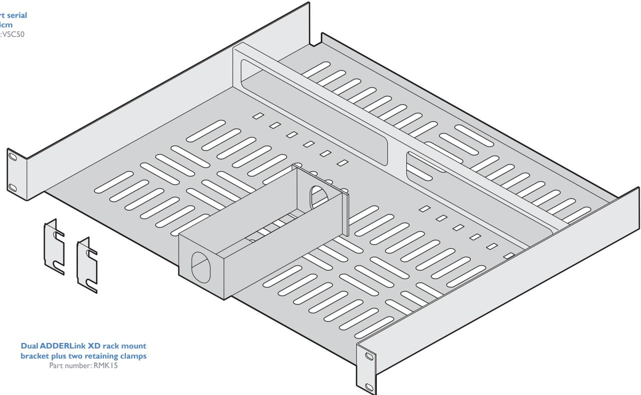
**Dual ADDERLink XD rack mount bracket plus two retaining clamps**
