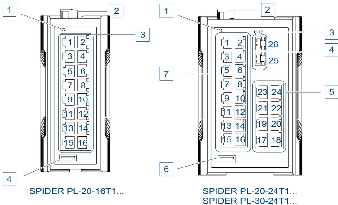
Front view using example of the device variants SPIDER PL-20... and SPIDER PL-30...
