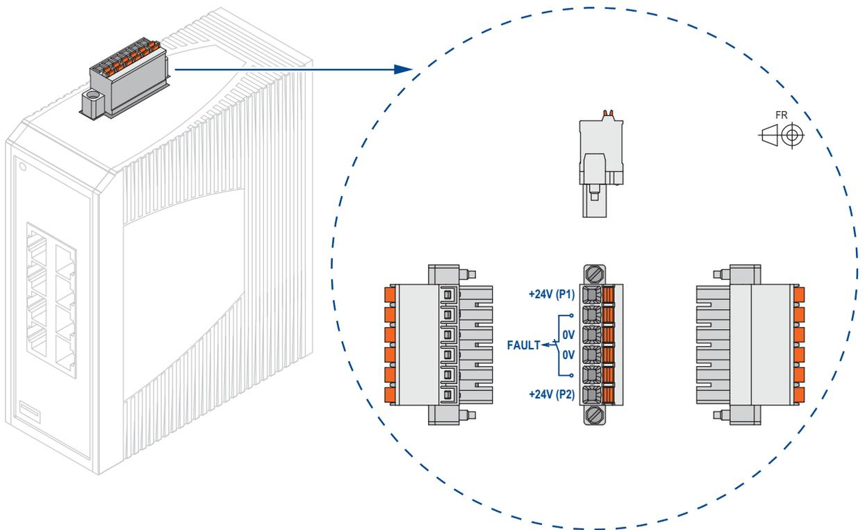
Figure 3: 6-pin voltage terminal with spring, characteristic value HK
